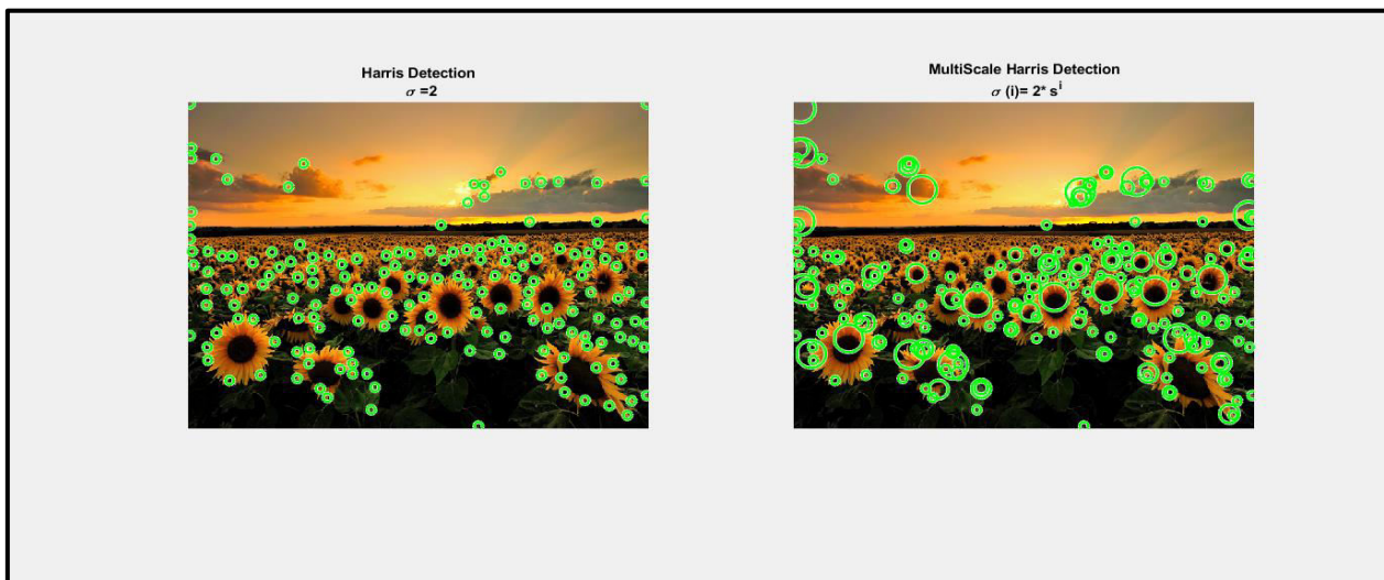
Fig. 1: Harris detection of corners with single scale and Multiscale Value of sigma.
