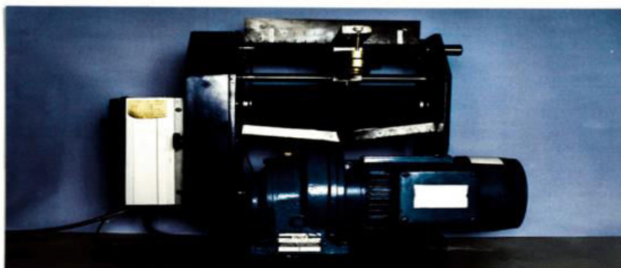
Figure: Photograph of the pin-on-drum machine
