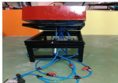
Fig.4- fig show actual view of multistage dumping trolley
