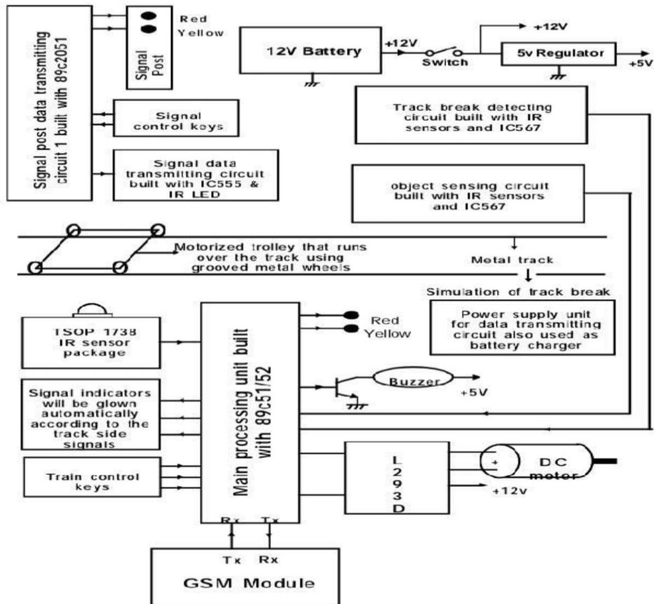
Fig.1. Block Diagram of proposed work
