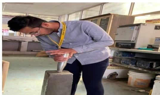
Fig.4 Column testing by using Rebound hammer
