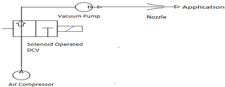
Fig 3: Pneumatic circuit for automatic seed sowing machine.
