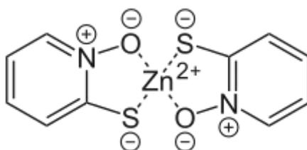
The pyrithione ligands, which are formally monoanions, are chelated to  $Zn^{2+}$  via oxygen and sulfur centers. In the crystalline state, zinc pyrithione exists as a centrosymmetric dimer (see figure), where each zinc is bonded to two sulfur and three oxygen centers.<sup>[3]</sup> In solution, however, the dimers dissociate via scission of one Zn-O bond. This compound was first described in the 1930s.<sup>[4]</sup>
