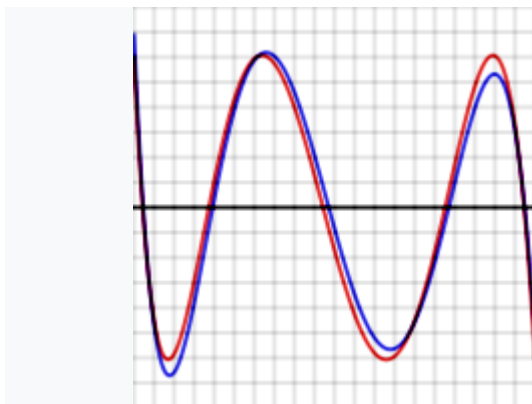
Error between optimal polynomial and \log(x) (red), and Chebyshev approximation and \log(x) (blue) over the interval [2, 4] . Vertical divisions are 10^{-5} . Maximum error for the optimal polynomial is 6.07 \times 10^{-5} .
