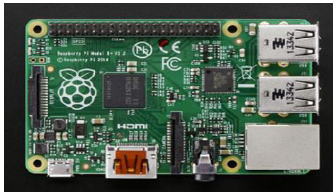
Fig.2. Raspberry pi model
