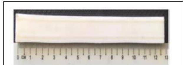
Fig.4 Flexural test specimens before testing
