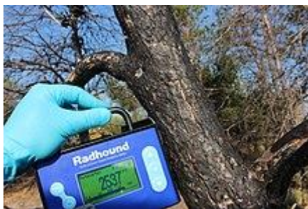
A Radhound Geiger counter measuring radiation emitted by a tree in Chernobyl
