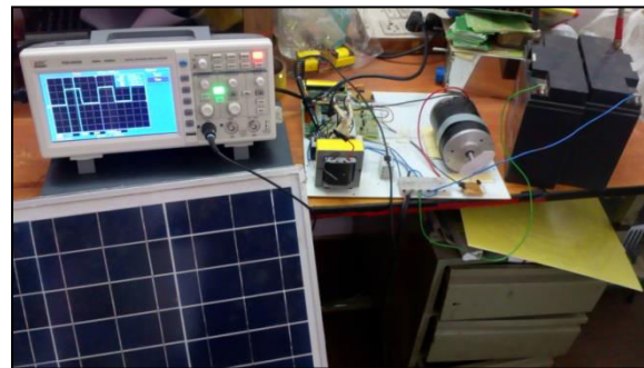
Fig 5.2: Hardware set up for solar PV fed DC motor speed control using microcontroller based power electronic controller
