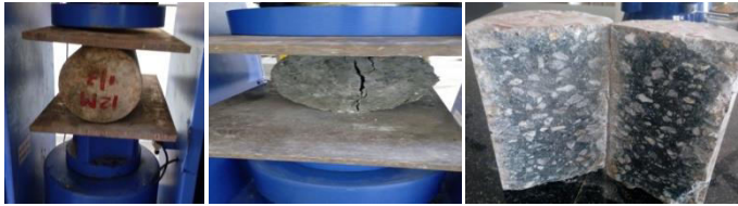
Figure 2: Split Tensile Test
