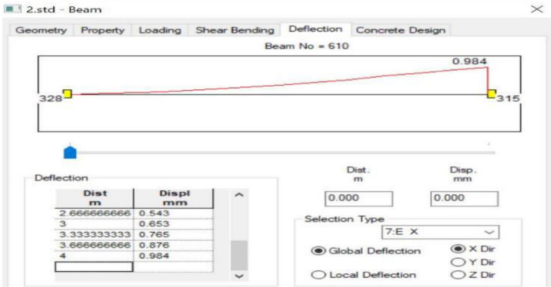
[Fig.4.3: Column deflection for medium soil]
